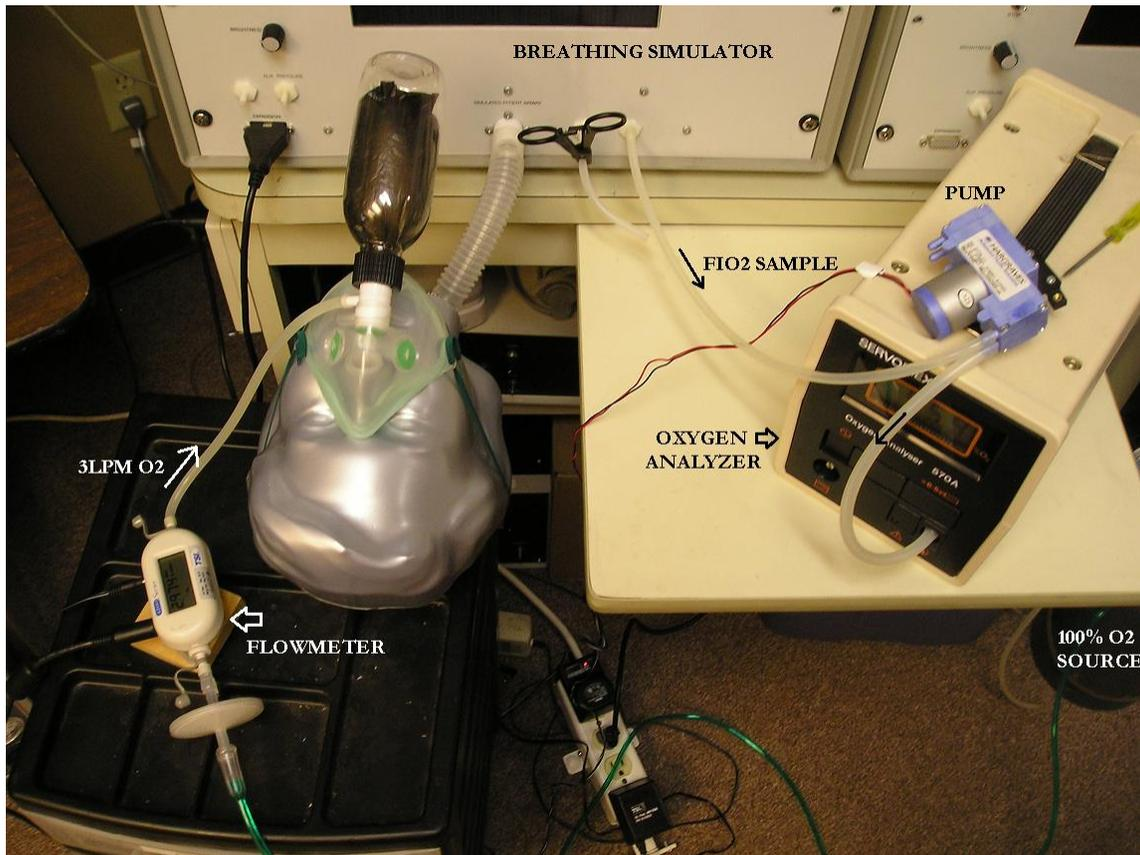
Silicone tubing was used to connect the breathing simulator sampling port to the pump inlet port, and also to connect the pump outlet port to the Servomex oxygen analyzer. The pump takes gas samples from the lung and directs them to the oxygen analyzer at a rate of approximately 0.725 LPM.
